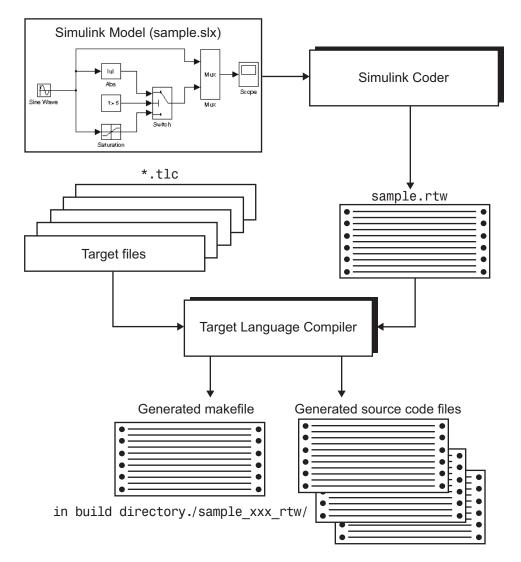
When generating code from a Simulink model, the first step in the automated process is to generate a *model*.rtw file. The *model*.rtw file includes the model-specific information required for generating code from the Simulink model. *model*.rtw is passed to the Target Language Compiler, which uses it in combination with a set of included system target files and block target files to generate the code.
