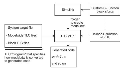
Just as a C program is a collection of ASCII files connected with **#include** statements and object files linked into one binary, a TLC program is a collection of ASCII files, also called scripts. Because TLC is an interpreted language, there are no object files. The single target file that calls (with the **%include** directive) other target files used for the program is called the entry point.
