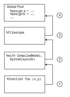
The rule for nested file scopes is similar to that for nested function scopes. In the case of nested file scopes, only the innermost nested file scope is searched.
