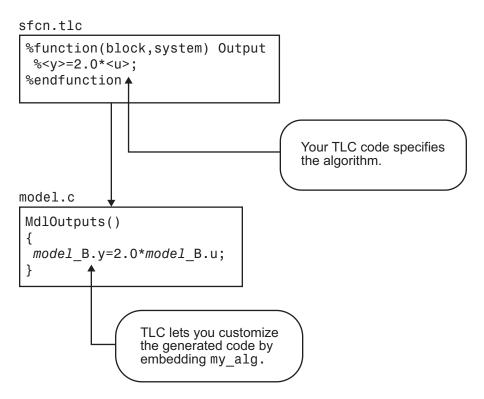
The S-function timestwo.c provides a simple example of a fully inlined S-function. This block multiplies its input by 2 and outputs it. The C MEX version of the block is in the file *matlabroot*/toolbox/simulink/simdemos/simfeatures/src/timestwo.c, and the inlining TLC file for the block is *matlabroot*/toolbox/simulink/simdemos/ simfeatures/tlc\_c/timestwo.tlc.
