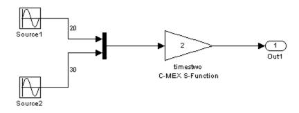
The input to the timestwo S-function comes from two arrays located at two different memory locations, one for the output of sourcel and one for the output of block source2. This is because of an optimization that makes the Mux block virtual, meaning that code is not explicitly generated for the Mux block and thus processor cycles are not spent evaluating it (i.e., it becomes a pure graphical convenience for the block diagram). So this is represented in the *model*.rtw file in this case as
