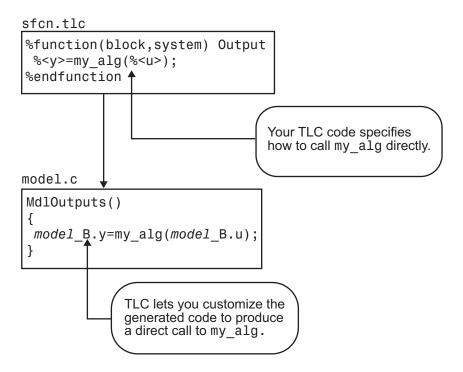
This is the inlining TLC file for a wrapper version of the timestwo block.
